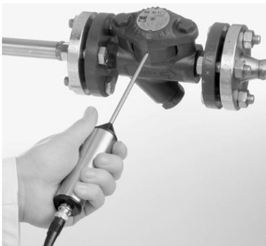
GESTRA Steam traps RHOMBUSline : Apply the tip of the probe laterally to the trap body.
